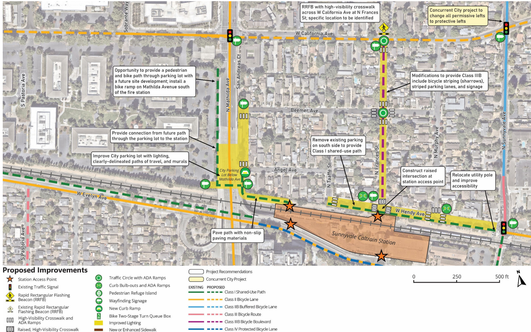
Figure 4: Overview of Recommendations, North of Caltrain
