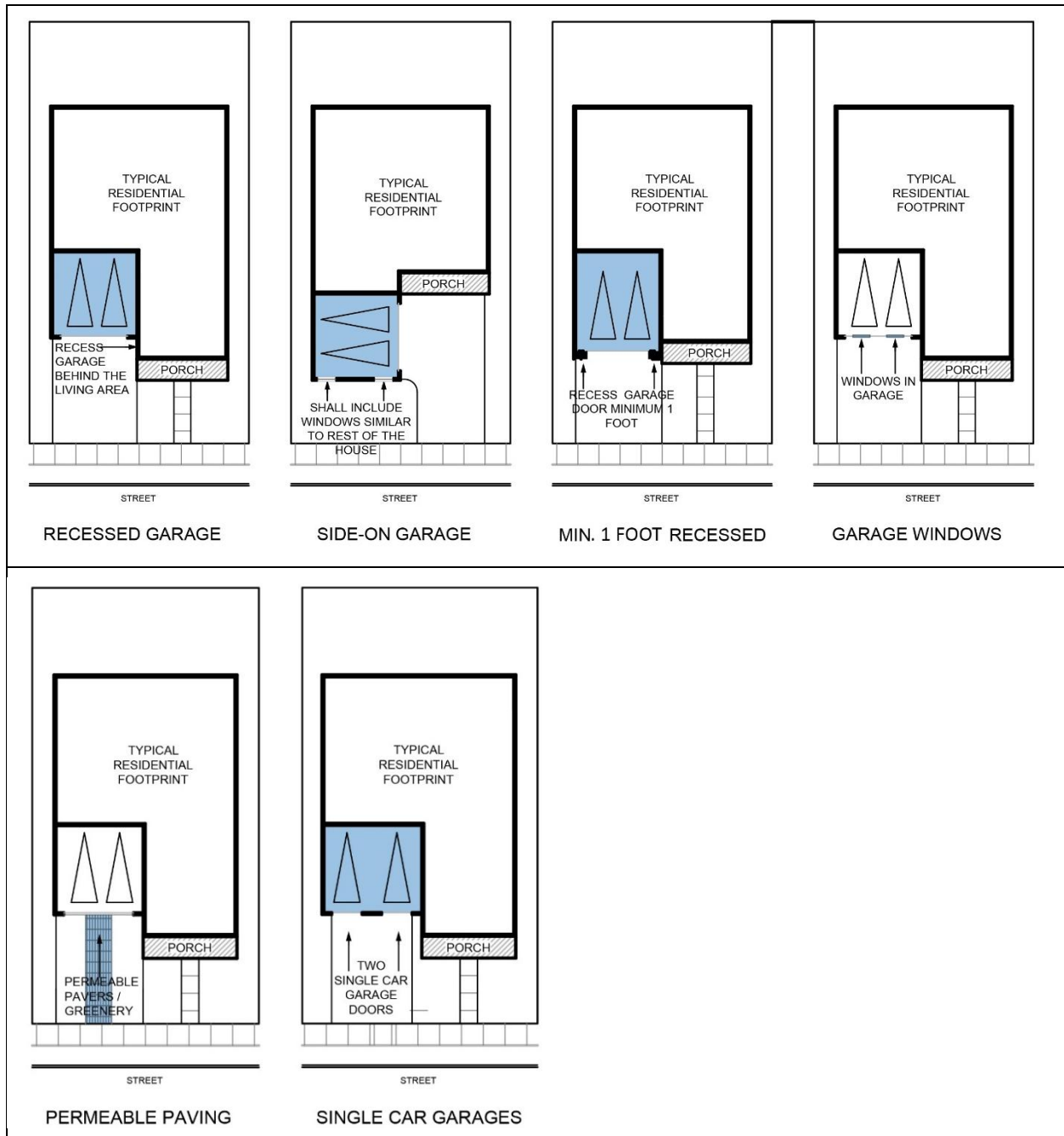
FIGURE 2.13: Examples of Garage Design Techniques
