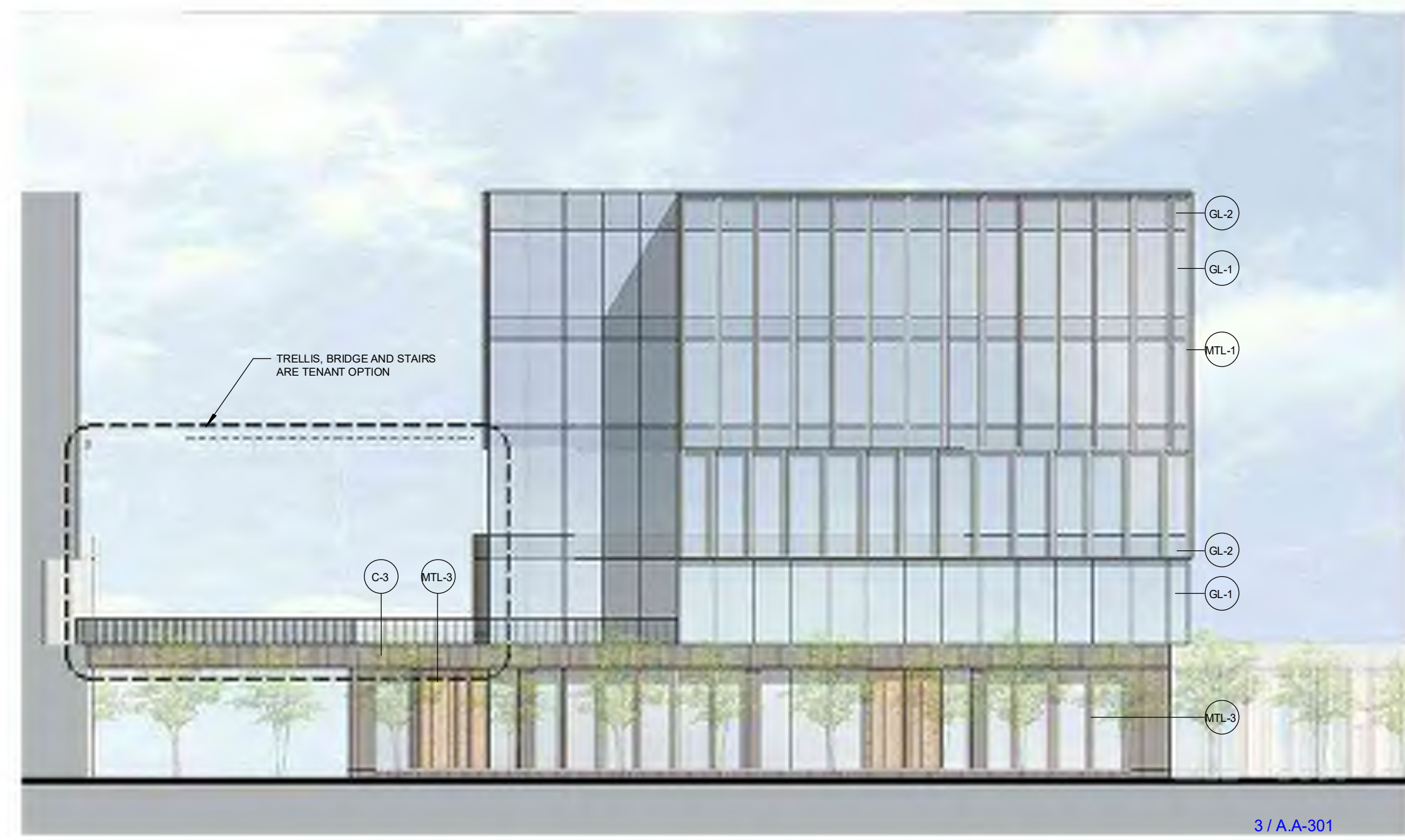
1 ELEVATION - BUILDING A - WEST 1/16" = 1'-0"
