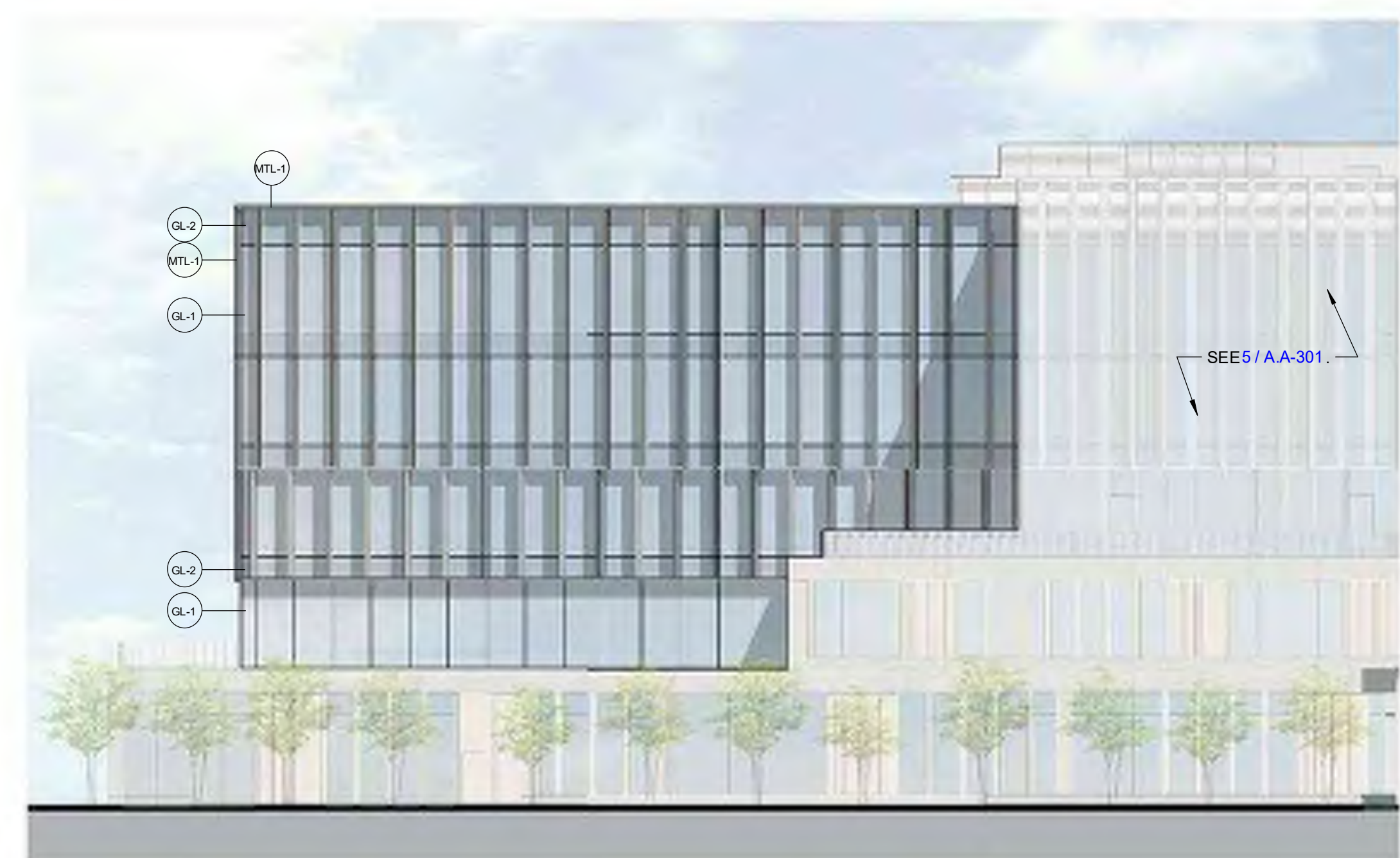
4 ELEVATION - BUILDING A - SOUTH (WEST WING) 1/16" = 1'-0"
