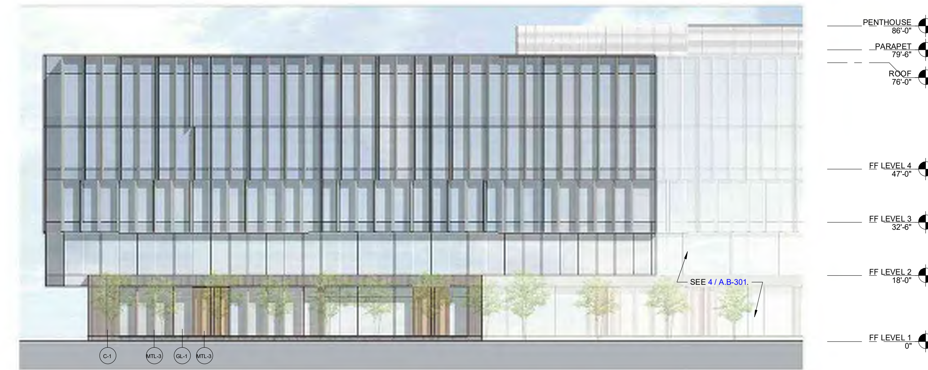
3 ELEVATION - BUILDING B - SOUTH 1/16" = 1'-0"
