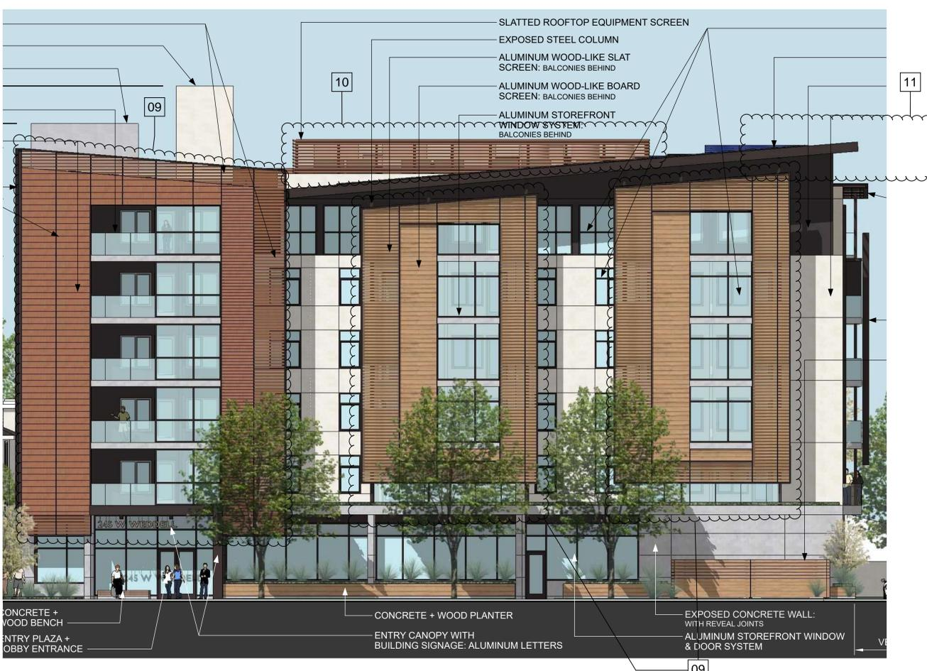
**2 SOUTH ELEVATION (STREET ELEVATION) - PLANNING APPROVAL DRAWING**
