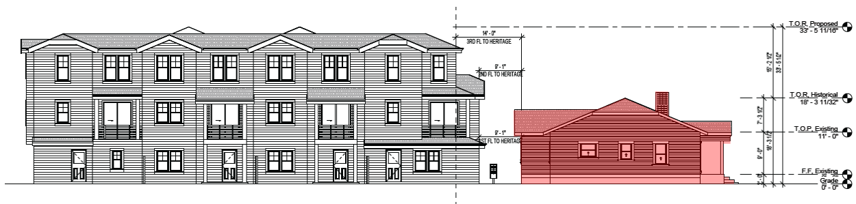
Figure 7: Proposed east elevation. The existing historic residence is shown at the right. The proposed new townhouse construction is at the left. Source: GKW Architects, 434 Crescent Avenue Residential Development, Sheet A201. September 2025. Edited by Page & Turnbull.
