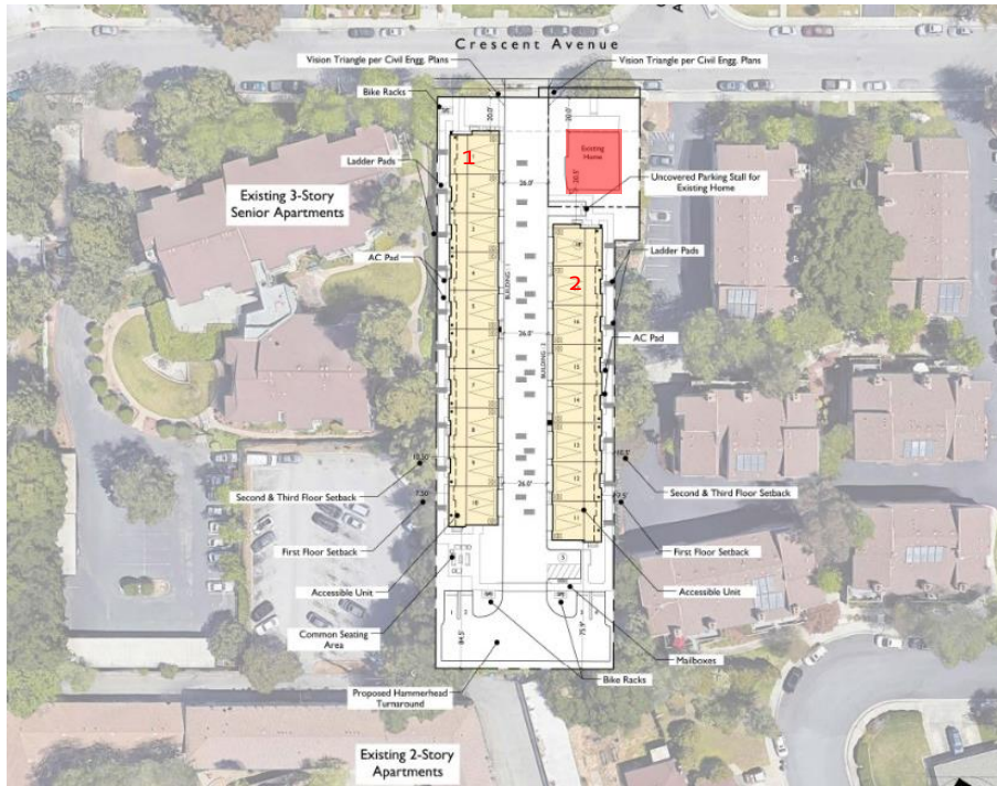
Figure 8. The proposed site plan with new buildings labeled in red, and the existing house at 156 Crescent Avenue blocked out in red (Bassenian/Lagoni Architecture, November 2022).
