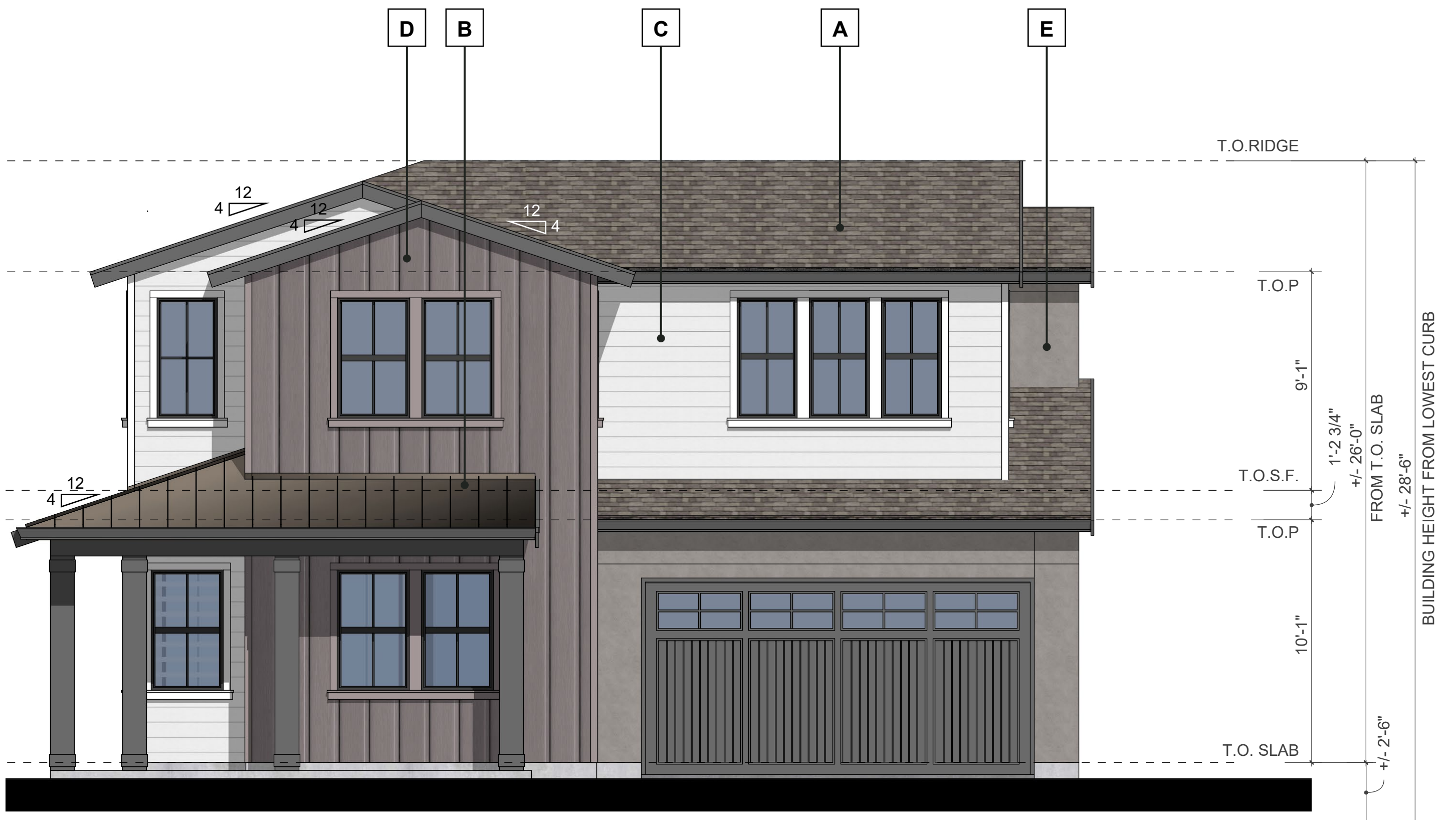
FRONT ELEVATION - TRADITIONAL CS1 LOT 1 LOWEST CURB 0'-0" (98.97' ALONG NORTHWEST LUSTERLEAF) SEE CIVIL SHEETS FOR CURB ELEVATIONS
