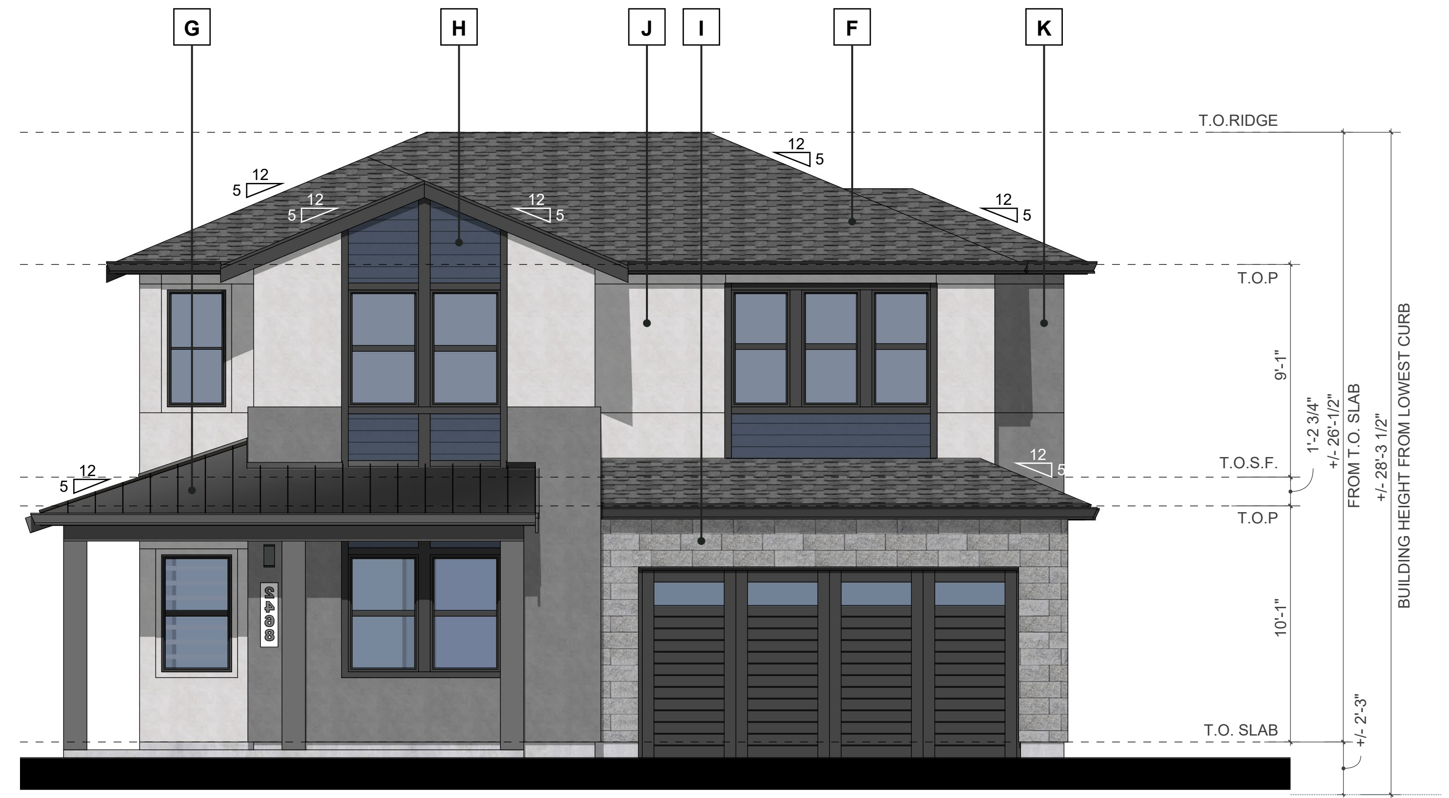
FRONT ELEVATION - MODERN CS1 LOT 8 LOWEST CURB 0'-0" (98.97' ALONG NORTHWEST LUSTERLEAF) SEE CIVIL SHEETS FOR CURB ELEVATIONS
