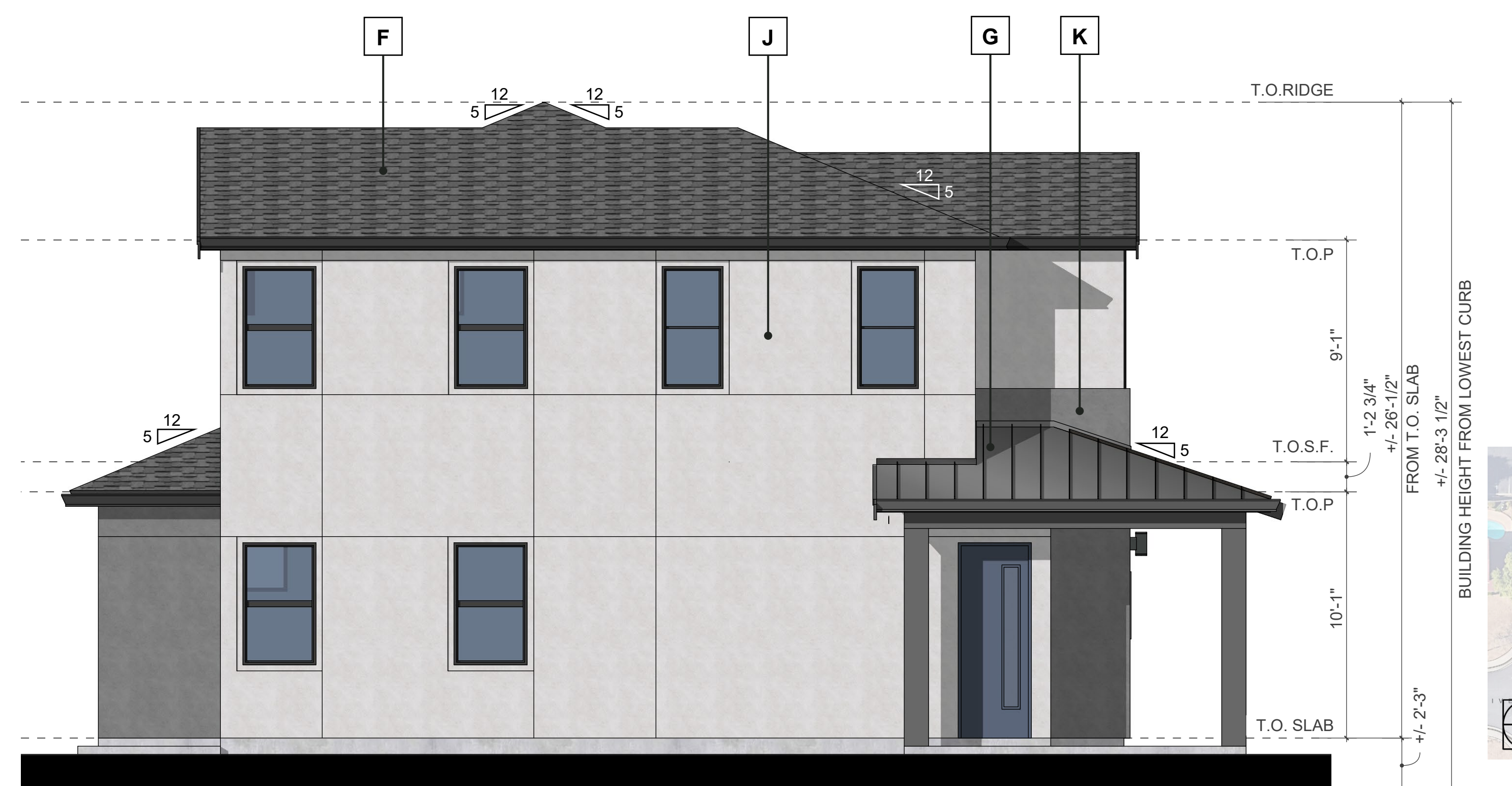
LEFT ELEVATION - MODERN CS 1 LOT 8 LOWEST CURB 0'-0" (98.97' ALONG NORTHWEST LUSTERLEAF) SEE CIVIL SHEETS FOR CURB ELEVATIONS
