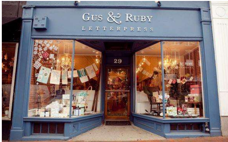
Above: Using one color for the storefront works here as the raised, simple letter signage at the sign band and the creative use of the window display area provides plenty of color and variation.
