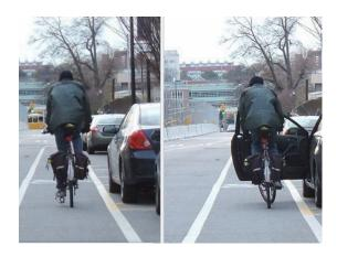
The lack of a buffer means no separation between bikes and moving cars. It also precludes protected bike lanes in the future. The zigzagging parking lane has parking zone transitions which tends to cause parked cars oozing into the bike lane at transitions (see photo below). This happens a lot on Wolfe, where parking zones start and end. Cyclists then have to dangerously veer around the parked cars into car traffic.
