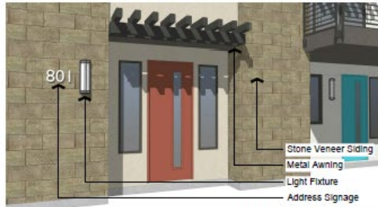
5. Unit Entry With Awning
