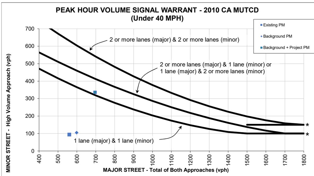
\* NOTE: 150 vph applies as the lower threshold volume for a minor street approach with 2 or more lanes and 100 vph applies as the lower threshold volume for a minor street approach with 1 lane.
