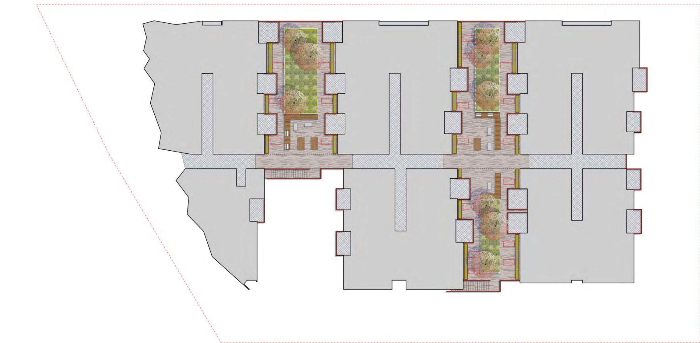
PLAY MOUNDS & ARTIFICIAL TURF RUBBER MOUNDS: - MANUF: TOT TURF - MODEL: SUPREME - 2" THICK Poured-IN-PLACE RECYCLED RUBBERIZED SURFACE ARTIFICIAL TURF: - MANUF: GRASS TEX - MODEL: PLAYTIME, PLAZA
