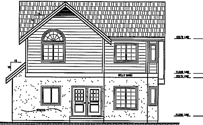
NORTH (REAR) ELEVATION SCALE: 1/8"=1'-0"
