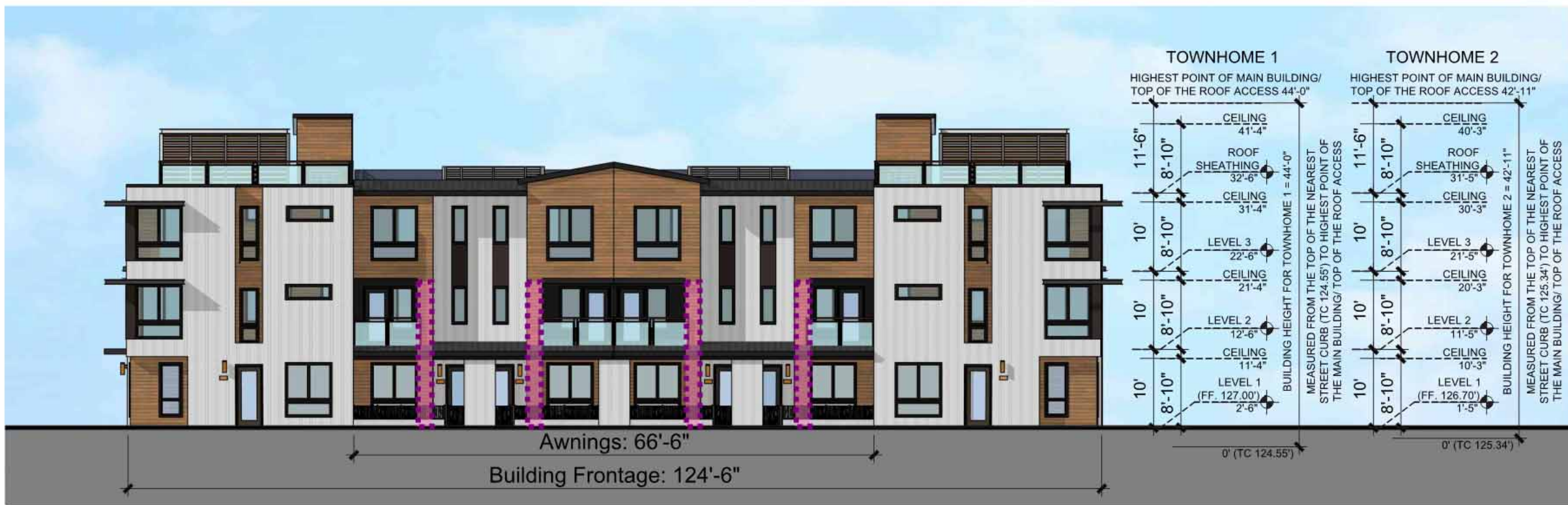
8-PLEX (TOWNHOME 1 & 2) FRONT EAST ELEVATION SCALE: 1/16" = 1'-0"
