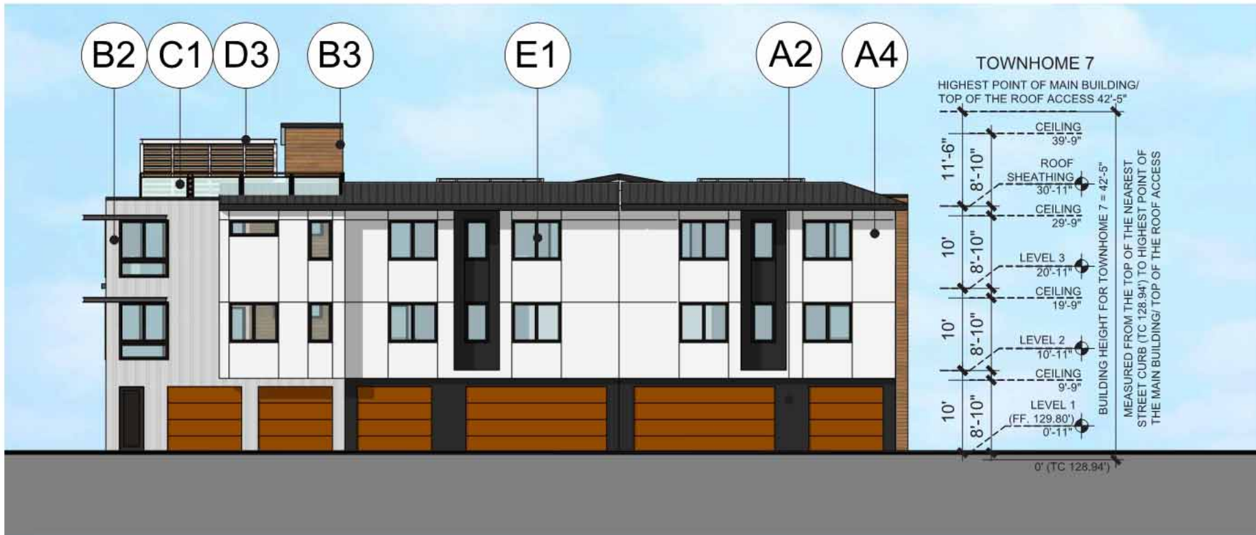
6-PLEX (TOWNHOME 7) REAR EAST ELEVATION SCALE: 1/16" = 1'-0"
