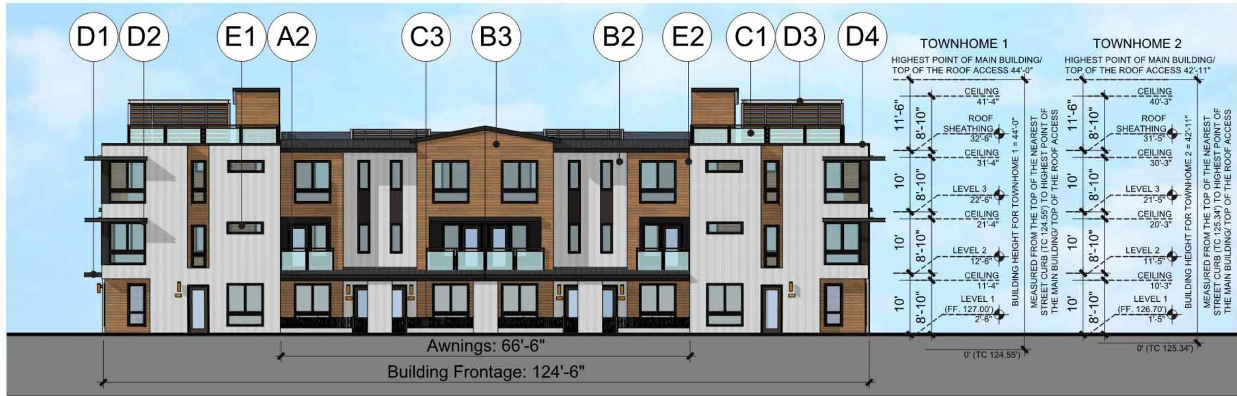
ECRSP 2.3.a_66'-6" / 124'-6" = 53.4% 8-PLEX (TOWNHOME 1 & 2) FRONT EAST ELEVATION SCALE: 1/16" = 1'-0"
