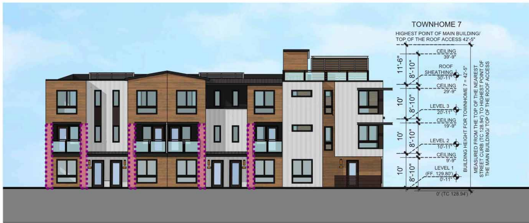
6-PLEX (TOWNHOME 7) FRONT WEST ELEVATION SCALE: 1/16" = 1'-0"
