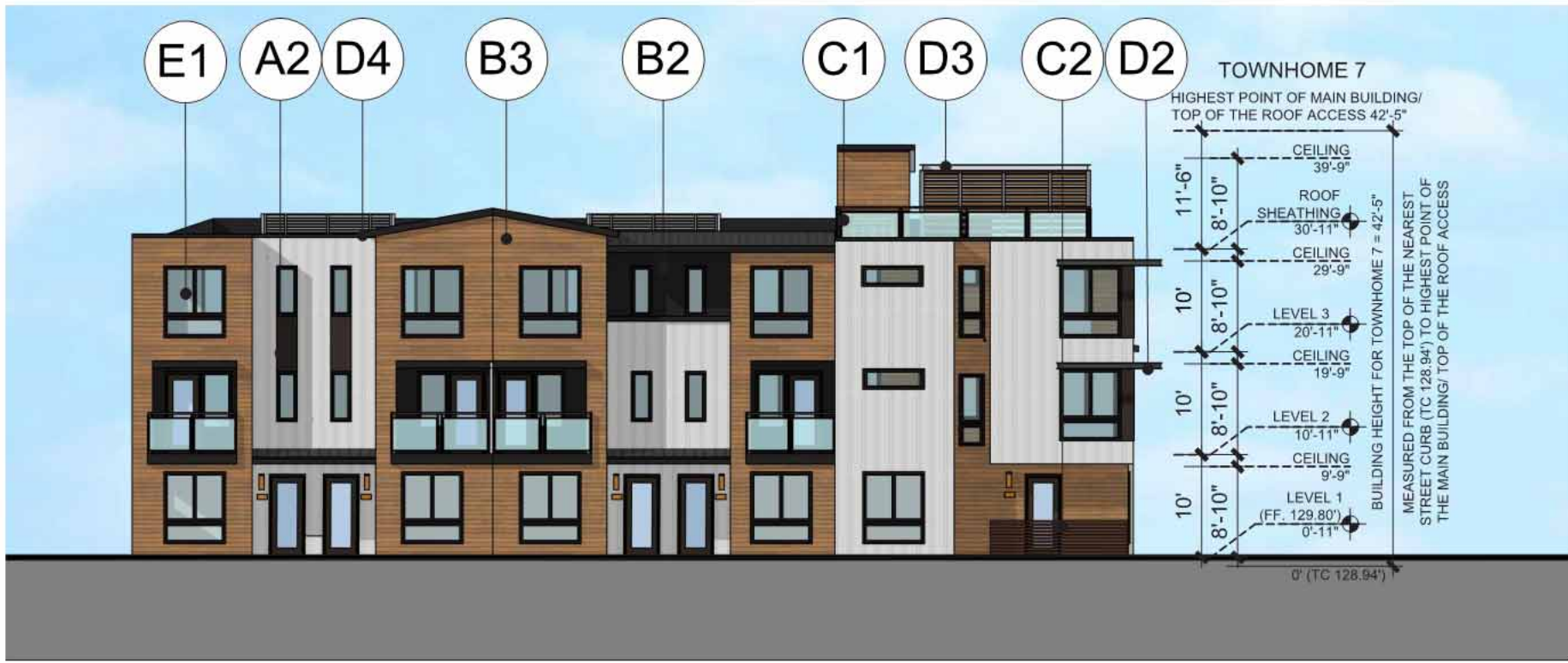
6-PLEX (TOWNHOME 7) FRONT WEST ELEVATION SCALE: 1/16" = 1'-0"
