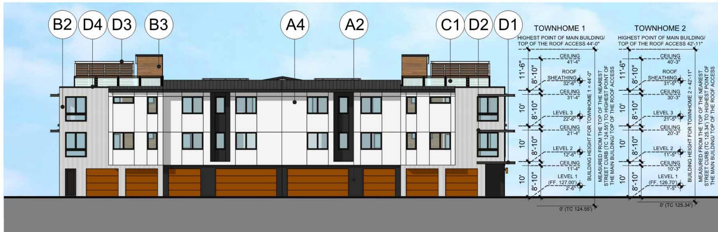
8-PLEX (TOWNHOME 1 & 2) REAR WEST ELEVATION SCALE: 1/16" = 1'-0"
