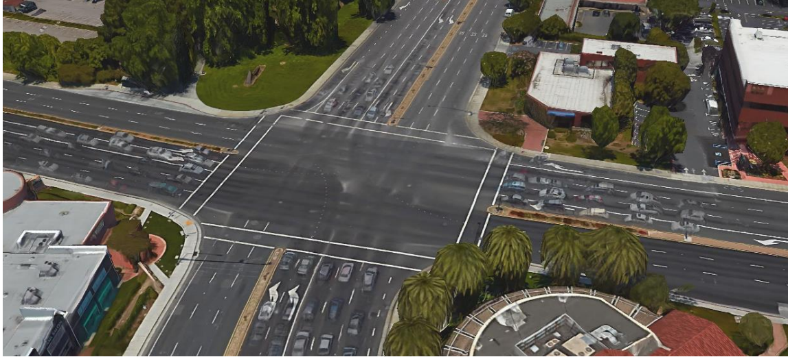
Figure B1. Street Configuration at Mathilda Avenue includes dual left-turn lanes and 125-foot crossing distance
