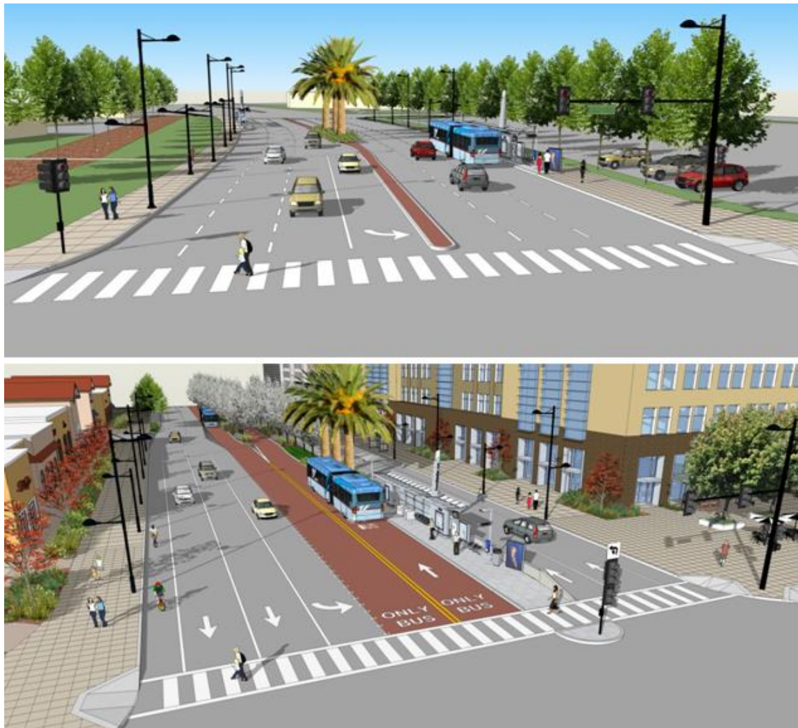
Figure B13. VTA BRT Concept Plans: Mixed Flow (top) and Dedicated Lanes (bottom)
