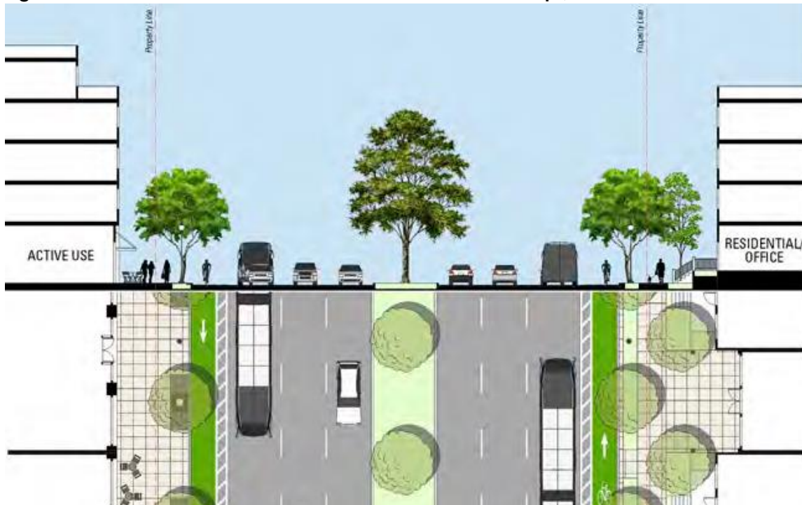
Figure B17. Mountain View El Camino Real Illustrative Concept, Bike Lane Variation
