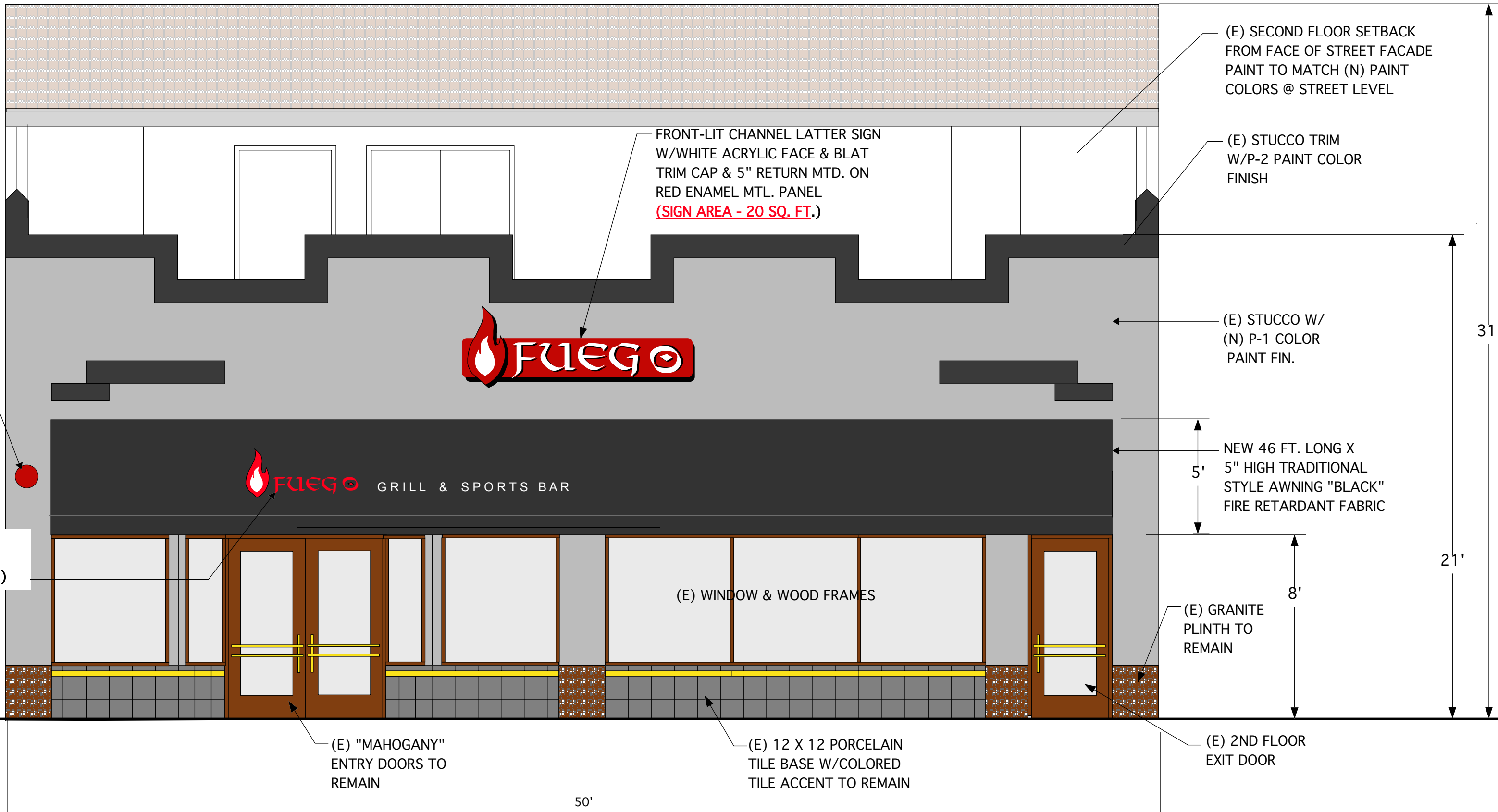
MURPHY AVENUE EXTERIOR ELEVATION SCALE: 1/4" = 1'-0"
