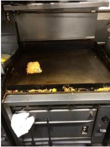
Figure 19 Doubletree Non-thermostatic Griddle
