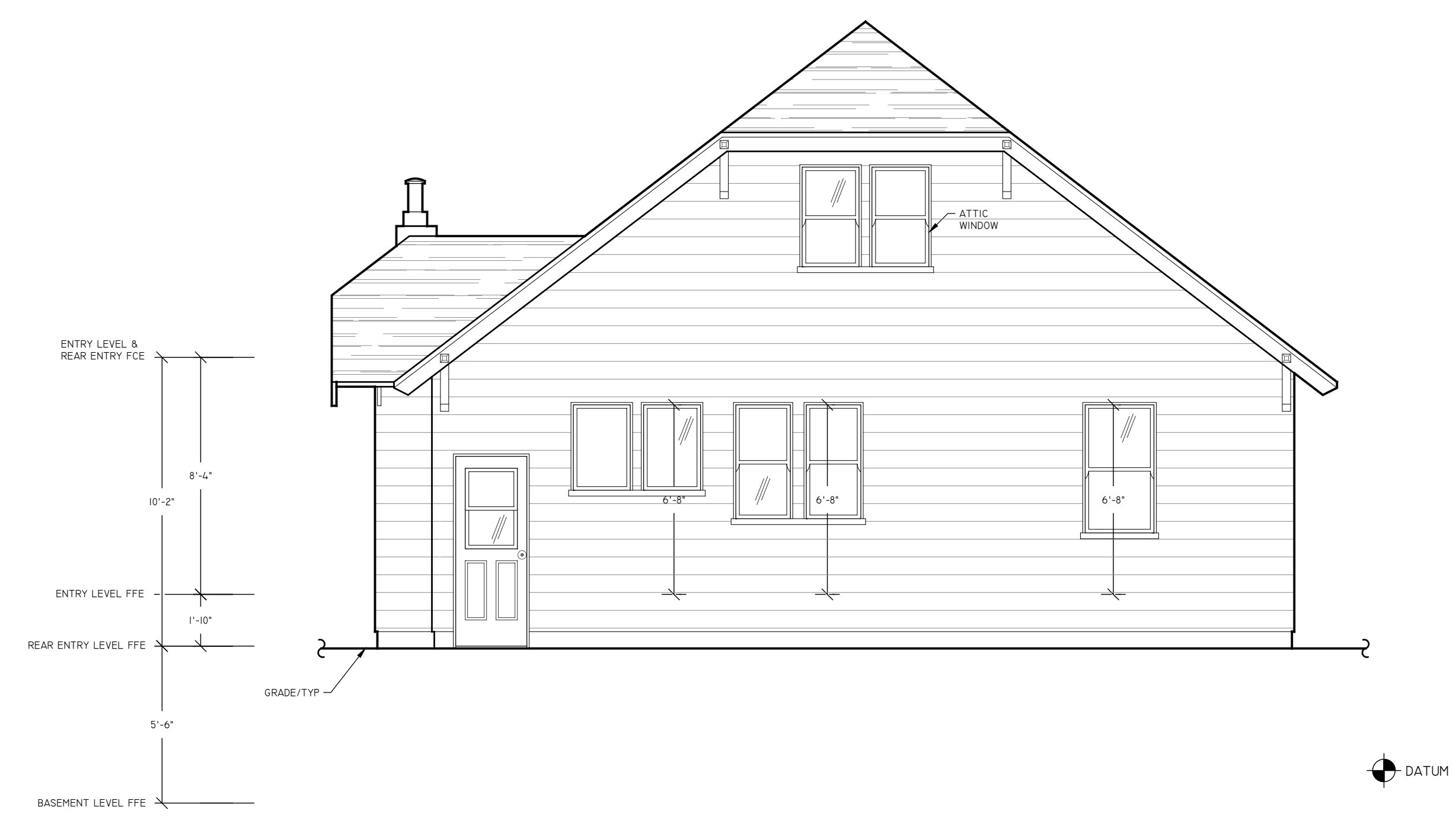
③ EXISTING SOUTH ELEVATION
