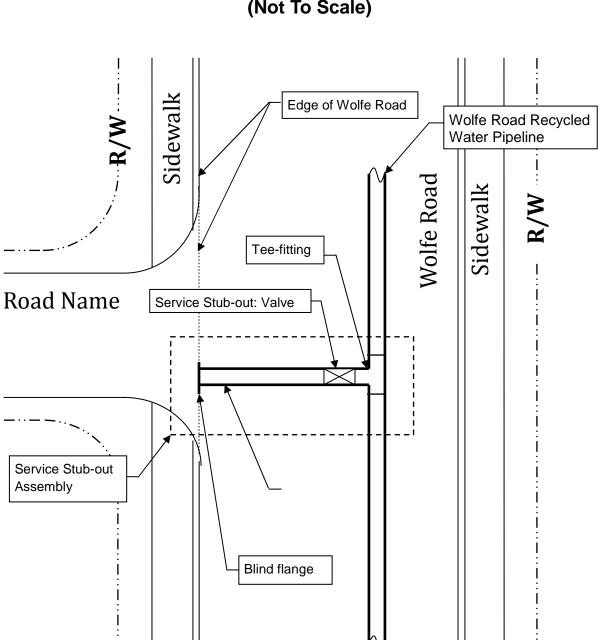
EXHIBIT B – EXPANDED VIEW OF SERVICE STUB-OUT ASSEMBLY (Not To Scale)
