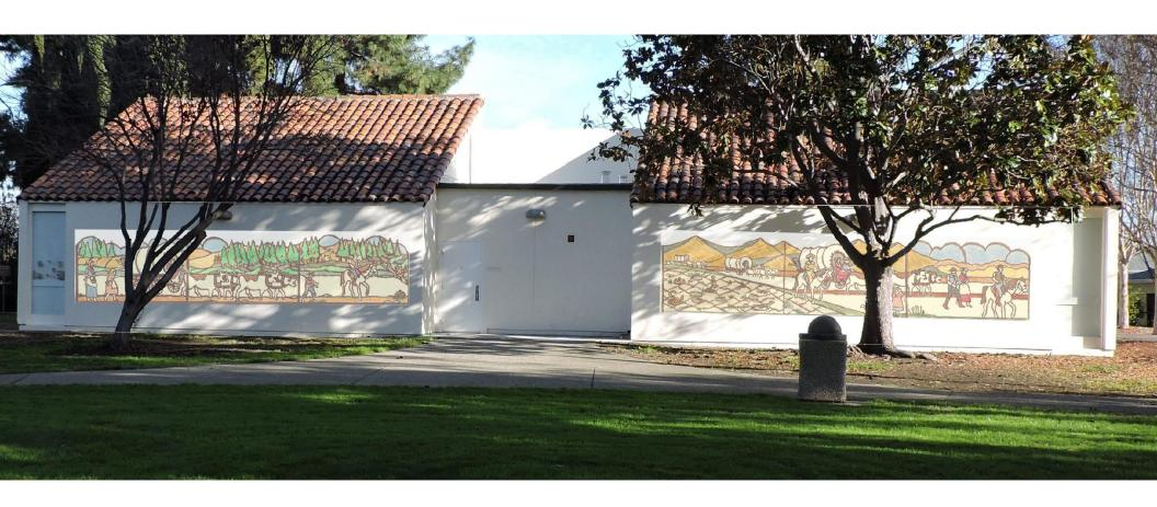
Elevation rendering of Sowell's design proposal. Each mural will measure approximately 24'w x 5'h x 1"d and be constructed of 1/8" metal sheeting. The metal sheeting will be cut so that the negative spaces of the designs are left, creating the "lines" of each scene. The lines will be painted a rust-brown and the bare wall behind the metal frame will be filled in with colored paint, reminiscent of a coloring book.
