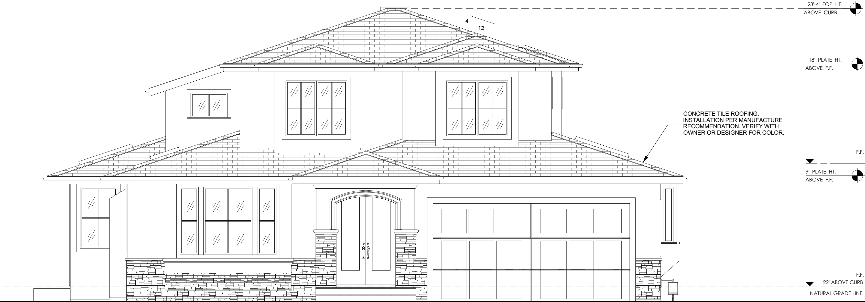
PROPOSED FRONT ELEVATION SC : 1/4" = 1'-0"
