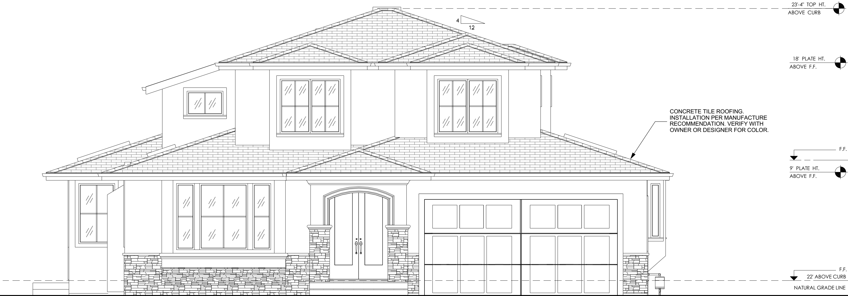
PROPOSED FRONT ELEVATION SC : 1/4" = 1'-0"
