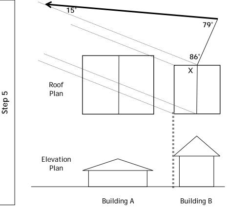
5. Draw a 79° angle from the end of Segment B. Find the point at which this new line intersects the shadow line. This creates a 15° angle - the altitude angle of the sun.
