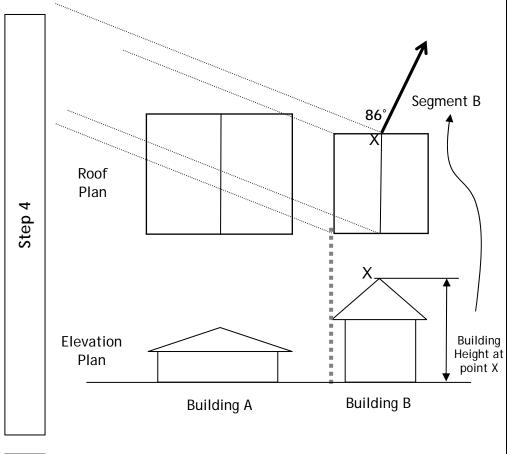
4. Choose one edge on the roof plan of Building B to draw the altitude angle. For this illustration, point X was used, but any roof edge may be used successfully. Draw a line segment ("Segment B") at an 86° angle to the shadow line at Point X (this will be parallel to the AM angle). The length of Segment B should be equal to the building height at point X, where Segment B is drawn.
