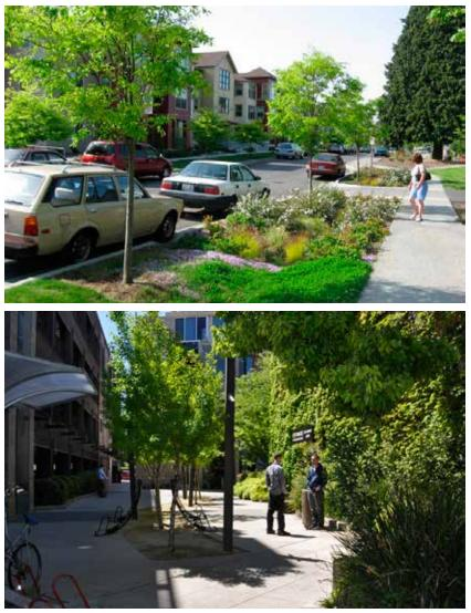
(Top) Bioswales along the street provide an attractive landscape with low water requirements while also assisting in drainage and stormwater management from paved surfaces. (Bottom) Trees and shrubs can add scale, help soften edges, and beautify pedestrian streets.
