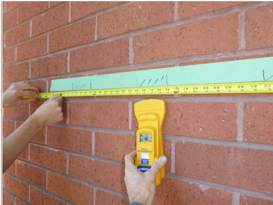
Photo 17: Scanning for rebar with Zircon MT6 metal detector.
