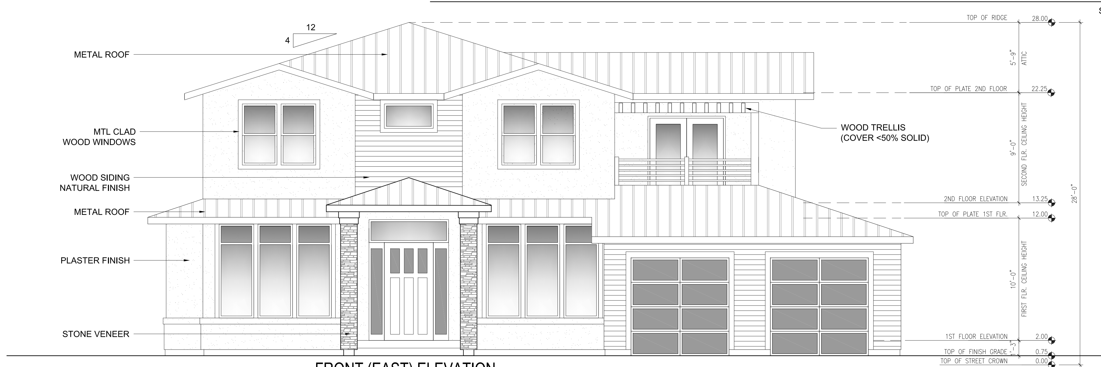
FRONT (EAST) ELEVATION
