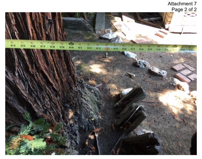
If you enlarge the picture, you can see that the edge of the tree falls at 5' from the fence. Per the drawing dimension, that would put the gas line 1' 3'' from the trunk, right below the roots.
