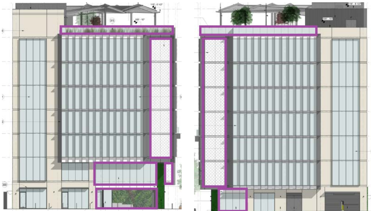
Figure 2. The extent of bird-safe glazing treatment to be incorporated on the east (left) and west (right) facades of the building is outlined in purple.
