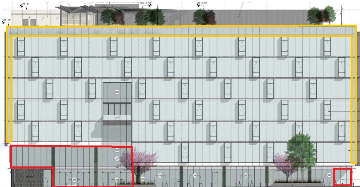
Figure 8. The north facade of the 100 Altair building. A free-standing glass ‘fin’ extends along the margins of the building’s north façade (shown in orange), posing a collision hazard to birds navigating around the building. Transparent glass corners that are located along potential flight paths for birds, and hence represent potential collision hazards, are shown in red.
