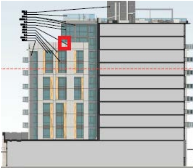
Figure 7. The north façade of Building 1 as seen from the Level 2 roof. A transparent glass corner that is located along a potential flight path for birds, and hence represents a potential collision hazard, is shown in red. In our opinion, this area should be treated with a bird-safe glazing treatment to comply with the City's guidelines.
