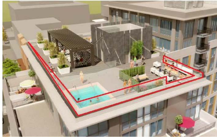
Figure 2. Free-standing glass railings extend along the margins of rooftops (an example from the roof of Building 1 is shown in red). Where these railings are located adjacent to landscape vegetation, they pose a collision hazard to birds that may try to fly towards landscape vegetation on the far side of the glass.
