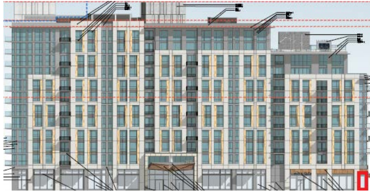
Figure 3. The west facade of Building 1 as seen from Taaffe Street. A transparent glass corner that is located along a potential flight path for birds, and hence represents a potential collision hazard, is shown in red. In our opinion, this area should be treated with a bird-safe glazing treatment to comply with the City's guidelines.
