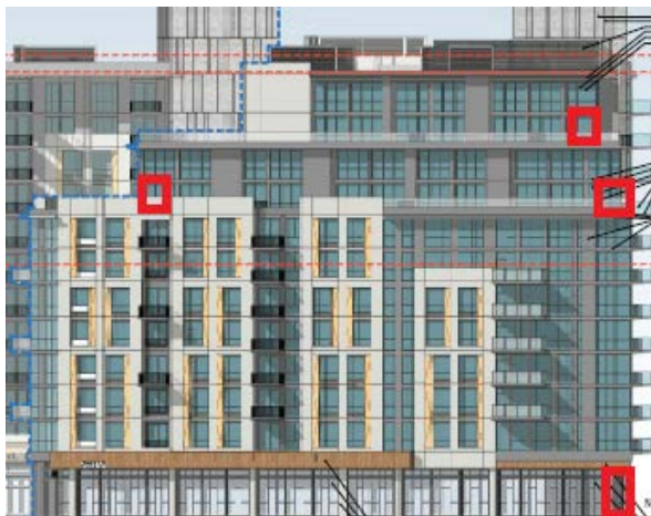
Figure 6. The east facade of Building 2 as seen from Murphy Avenue. Transparent glass corners that are located along potential flight paths for birds, and hence represent potential collision hazards, are shown in red. In our opinion, these areas should be treated with a bird-safe glazing treatment to comply with the City's guidelines.
