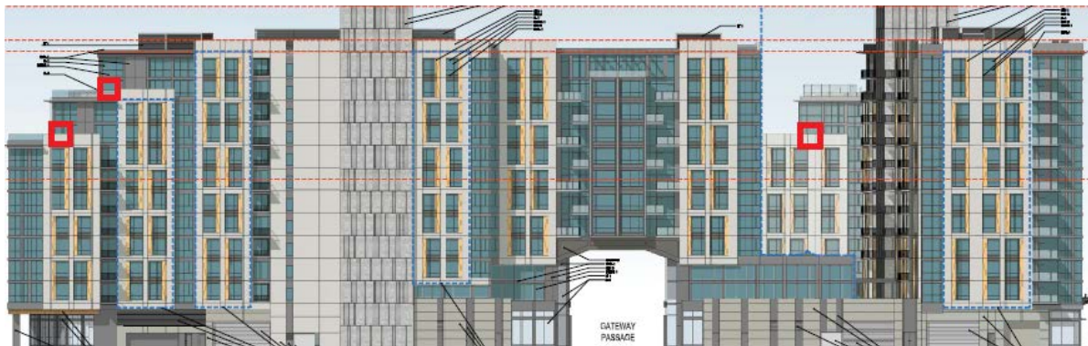
Figure 4. The north facades of Buildings 1 and 2 as seen from New Street. Transparent glass corners that are located along potential flight paths for birds, and hence represent potential collision hazards, are shown in red. In our opinion, these areas should be treated with a bird-safe glazing treatment to comply with the City's guidelines.
