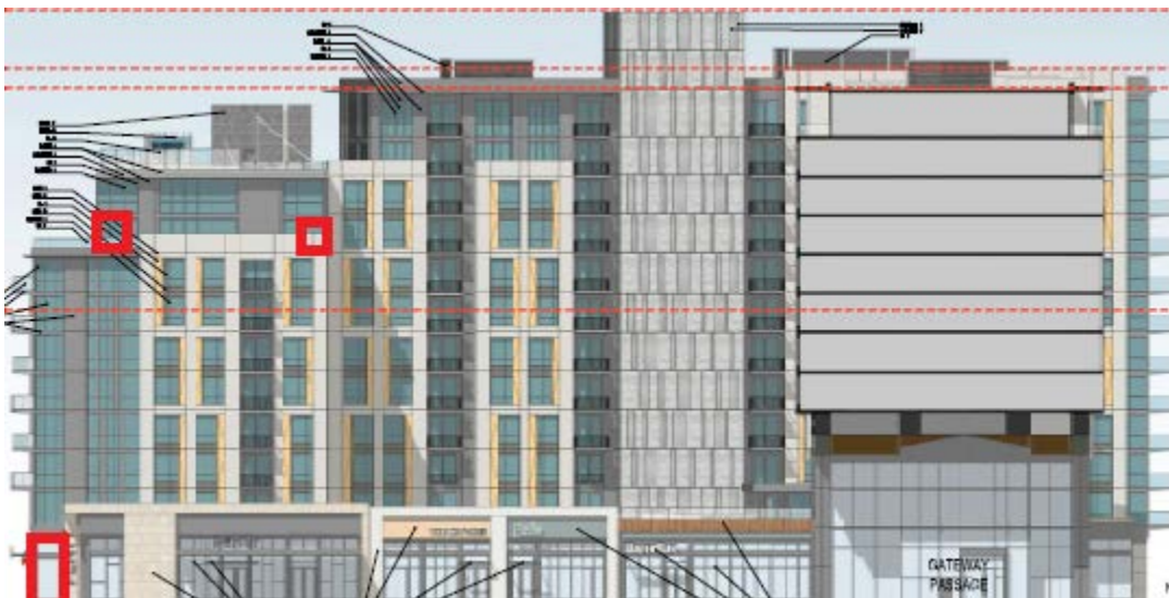
Figure 9. The east façade of Building 1 as seen from the public plaza. Transparent glass corners that are located along potential flight paths for birds, and hence represent potential collision hazards, are shown in red. In our opinion, these areas should be treated with a bird-safe glazing treatment to comply with the City's guidelines.
